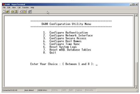
2. Type 2 and press Enter to select 2. Configure Network Interface. The Network Interface screen displays.
